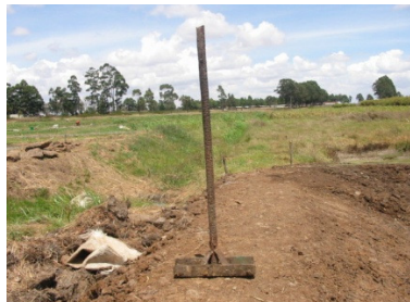
14: A simple and inexpensive soil compactor made from scrap metal (Mbugua H. M.)
